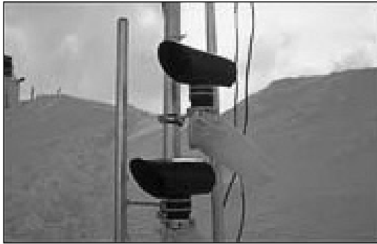
Fig. 3: Top left - Prototypes tested in wind tunnel, at LASEN-EPFL. The acoustic response of cylindrical and spherical forms excited by wind were characterised in the 0 - 12.5 m/s range (from Th. Castelle). Top right - Calibration with controlled particles flux on test-bench, at LEMA-EPFL. (from Th. Melly). Bottom - Prototype tested at Anzère ski resort (2400 m).
